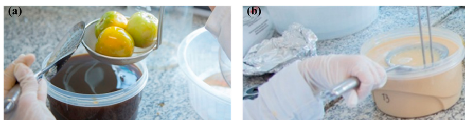
Figure 2. Detail of carnauba wax emulsion appearance for nanoemulsion (CWN) (a) and milky appearance for conventional carnauba wax (CWM) (b).
